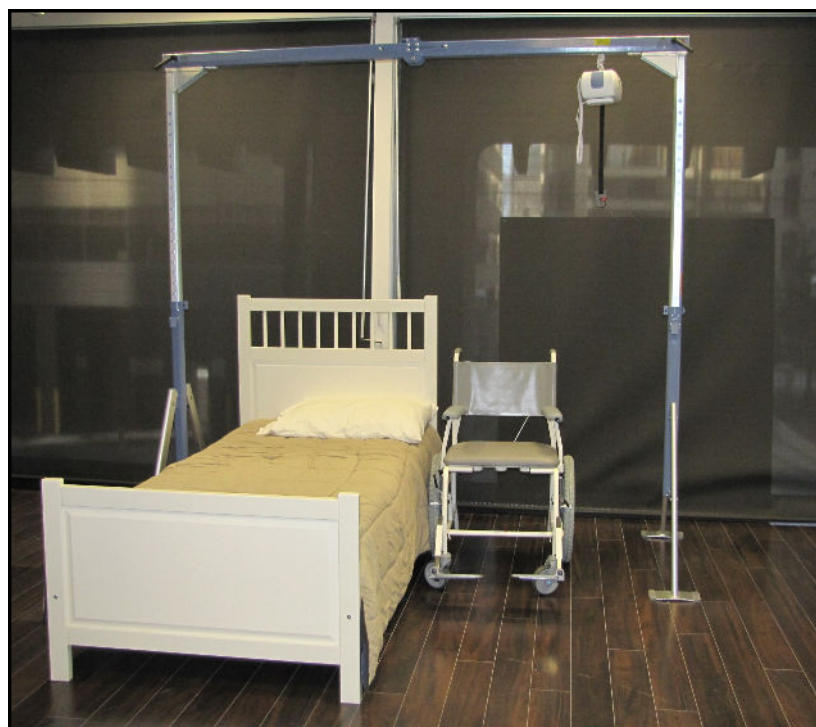
Completely Installed Free Standing Track
