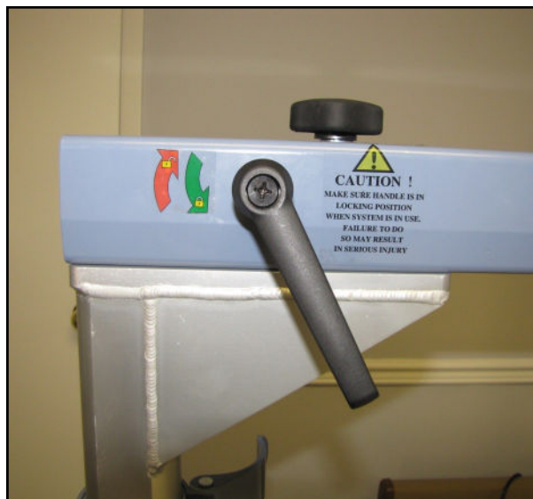
Note: Above picture shows that the plastic knob is flush with track, and track locked with top post.
