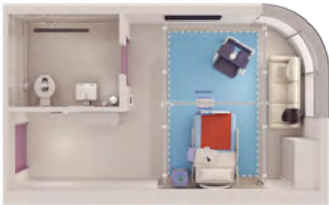
A single traverse track bariatric X-Y system covering bed with extended fixed tracks providing coverage between foot of the bed and wall for rehab purposes...
