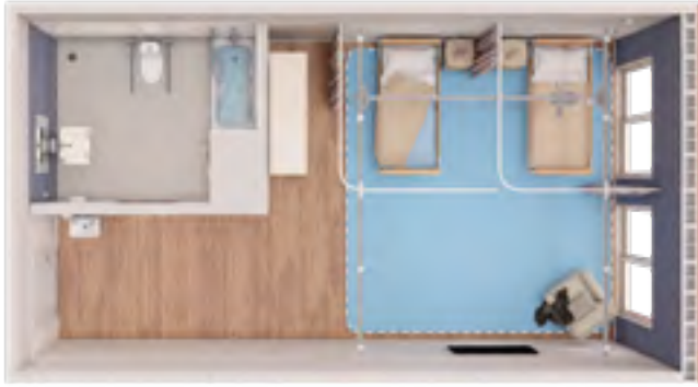
X-Y system covering two beds with extended fixed tracks providing coverage between foot of bed and wall for rehab purposes. Gaps in fixed tracks, maintain patient privacy, permitting the curtains to pass through.
