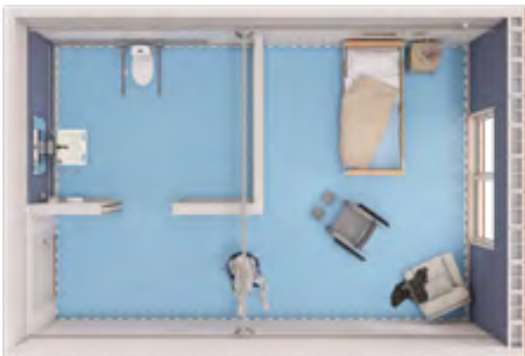
Wall mounted. X-Y tracking solution covering the entire living area, lowered bathroom walls permitting the traverse track of the X-Y system to travel above the walls.
