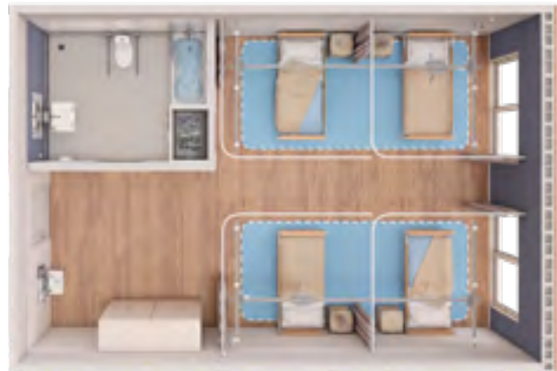
Ceiling mounted. Two separate X-Y tracking solutions, covering each side of the room. For fixed or portable ceiling lifts.
